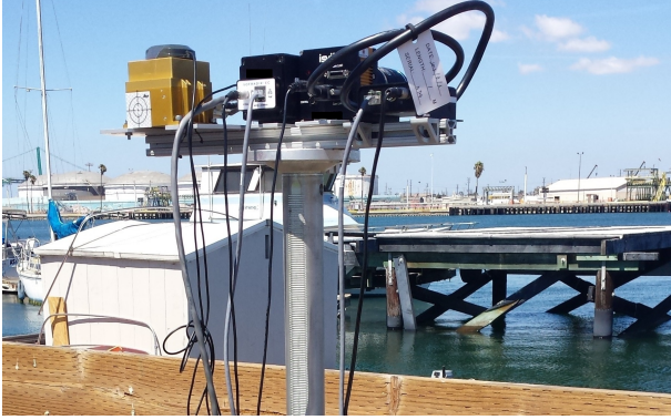
Figure 2. Our multi-modal stereo camera rig collecting data.
